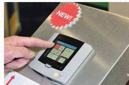
The new wireless Whale iVan Smart Controller calculates the amperage draw; you can set the maximum you want to apply.
