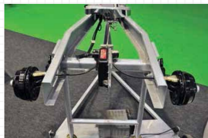
AL-KO's ATC stability system applies the brakes if the caravan starts to sway; it's especially valuable when towing in winter.
